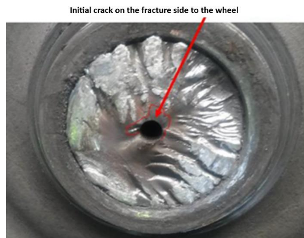
Fig. 6. Position, shape and structure of the initial crack to the drive wheel
