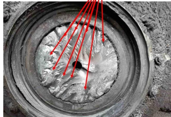
Fig. 9. Relief of the tearing structure in the drive locomotive shaft on the side of the reducer
