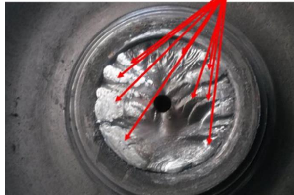
Fig. 10. Relief of the tear fracture structure on the drive locomotive shaft on the wheel side
