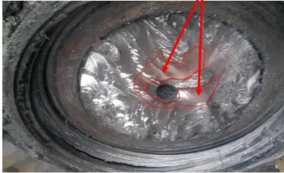
Fig. 7. Propagation of the initial crack in the shaft, position on the side of the resulting fracture to the reduction gear
