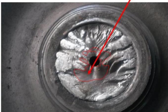
Fig. 8. Propagation of the initial crack in the shaft, position on the side of the fracture to the drive wheel
