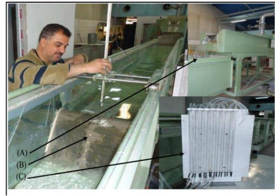
Fig. 9. A) The channel used in the experiments has triangular Sharp, B) stepped spillway model, and C) a piezometer board [37]
