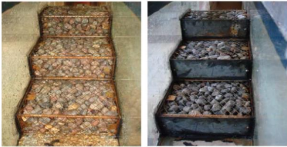
Fig. 14. Sketch pooled stepped spillway was used in the study [56]
