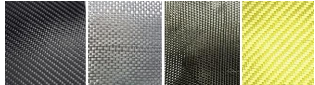
Fig. 9. Different fibrous polymers: CFRP, GFRP, BFRP and AFRP
