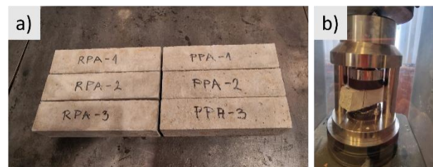
Fig. 1. Experimental setup: a) specimens for testing the pozzolanic activity of ash, and b) compressive strength testing [33]
