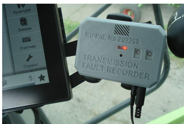
Fig. 6. In-cab transmission fault recorder for a combine harvester
