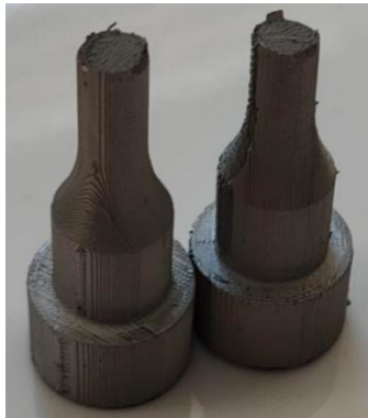
Fig. 4. Specimens after tensile testing
